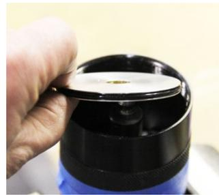
With the upper shaft and piston plate removed, you will see the lower piston plates sitting just below a large snap ring. Remove the snap ring. NOTE the position of the lower piston plate. It is actually sitting in the snap ring groove. When reinstalling the lower piston plates, DO NOT push this plate "below" that groove. The snap ring groove is wide enough to accept both the plate and the snap ring.
