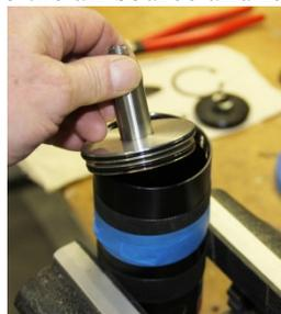
Once the piston shafts and plates have been removed, clean the inside of the power pack housing to remove any residual debris and lubricate it with a small amount of light machine oil.
